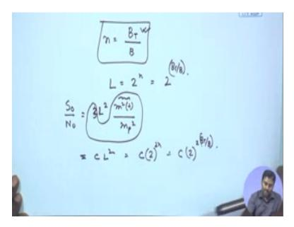
So this is my effective bandwidth model and which could be occupying the channel and this is the base that means actual signal bandwidth okay so this what I require now we want to go back to the relationship between L and m and n so l is  $2^n$  or I can write 2 d2 /d3 what happens to my signal to my noise ratio we have already represented signal to noise ratio as  $3l^2 m^2 t /mp^2$  this 3 and these things if you just make them constant.
