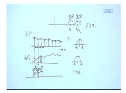
So basically suppose the multiplex was one of the important thing that was required for our transmission so we have said that suppose I have multiple signals okay and I want to simultaneously transmit that over a same media so let us say here is the media or if I have a wired media so everybody wish to actually simultaneously communicate through that same media okay so this is something we have done in amplitude modulation or even frequency modulation, so or general modulation theorem.
