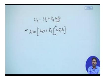
Okay, so what we have started exploring is the frequency output of the oscillator we are targeting which is we have proven that that should be  $\omega$  C into KF into MT, we have defined what is  $\omega$  C and what is KF okay. So this is something we have already discussed right. Now FM generation once we have this circuit that means our particular oscillator with an inductor which is fixed and a very cap where it varies with the input that bias voltage okay.
