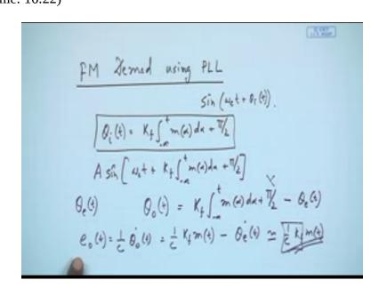
There is another way that is FM demodulation using PLL. So if you remember that for PLL we have also used a VCO right that was how we have designed TL. So for FM modulation we have already used VCO, now for demodulation also we will be just using PLL and PLL also as VCO in it. So basically FM modulation demodulation both will have key component as the VCO so once you have VCO you can do both modulation demodulation if we can appreciate this particular circuitry.
