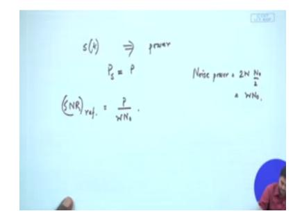
So this s(t) corresponding power or Ps that is actually P / P is the way it is defined P corresponding power spectral density if you integrate from- W to + W that is something you could okay. So now we know the power of it at the modulated, so therefore the baseband also must transmit that same power P fortunately here we are getting exactly and power okay. So if I just transmit empty whatever power it will be that is the same power we are getting okay.
