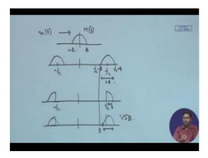
And if I wish to do that the corresponding filtering you can see that might have a nice roll off because I do not have to do a sharp cutoff at that frequency so this is called the VSP or we call it vestigial sideband okay so it's a little bit distorted sideband we are taking and we are actually taking a mix of both side band both way distorted but you will see that will in such a way we will design the filter so that we can actually get back the original sign alright.
