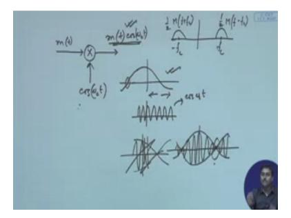
So basically it will be just centered around FC and that same criteria will be coming that this will be MF - FC this will be MF + FC and of course with half, so it will be centered around FC, so this is the frequency domain representation and the corresponding time domain representation we have understood from this particular thing that it is carriers whose amplitude is instantaneously varying with respect to the message signal which is a slow varying signal according to our assumption.
