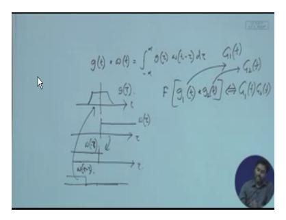
Something called convolution I am not going to prove that but I will just state what do we mean by convolution so this convolution is given by this \* symbol so that means the signal is convoluted with another signal GT is convoluted with another signal WT what does that means convolution actually means this so what is happening so you take this signal GT now is just do not worry about  $\tau$  that the dummy variable of in this integration okay.
