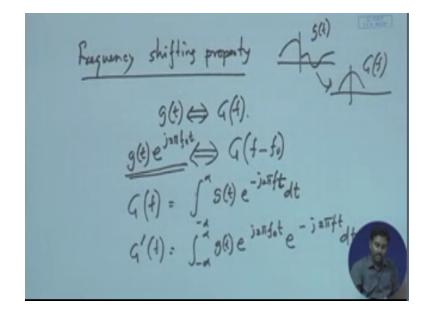
And I know the Fourier pair of that if I multiply that signal with e to the power  $J2\pi F_0 T I$  get our frequency shifting or frequency translation by an amount  $F_0T$  whichever exponential I am multiplying by okay so basically what happens the shape remains the same it just gets translated so now let us try to see what is the implication of this thing okay the biggest implication is suppose I have a signal G (t).
