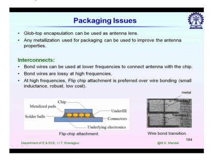
So here it showing a typical flip chip attachment in the right hand side left hand we have CPW line so left to right it is being connected by wire bonding. Any metallic wire if I we use some bend it is associated with inductance and wire bonding it is always forms a part of a loop.
