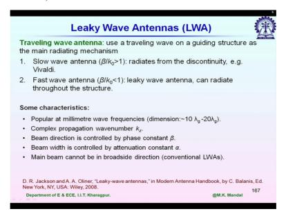
Some basic characteristics since these structure it leaks power throughout its length so we have to use the complex propagation wave no KZ. We have both alpha part and beta part it will be basically a wave guiding structure with some sort of semi open or open structure so that it can radiate or leak power throughout its length then the alpha part its non zero for the guiding structure. Beam direction is controlled by phase constant beta.
