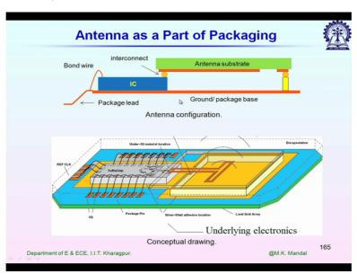
So finally how it looks when we for integration? This is a scheme suggested by IBM so let us say we have the integrated circuit here on silicon then antenna it is being fabricated in laminates so this is not on chip antenna but antenna as a part of packaging and the antenna radiator is connected to MMIC by using flip chip attachment in this particular example. And right hand side you can say we have a support for the substrate it cannot hang in air.
