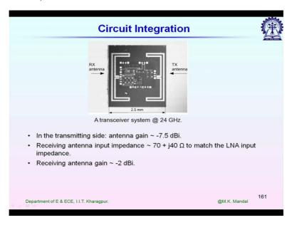
Typical this is 1 example. We are using 2 folded loop. 1 for the receiving side another for transmitting side and you see 1 interesting thing the antenna gain for the transmitting side is just minus 7.5 DBI while for the receiving side it is minus 2 DBI. Why so? This is due to the coupling between the circuit plot and the antenna radiator here. They are not using any guard ring or any precaution.
