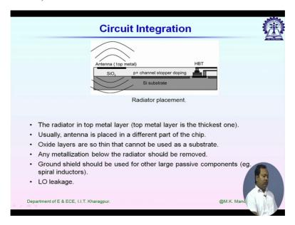
The some other issues when we go for circuit integration. Radiator it should be placed on top metal layer for gallium arsenide fabrication is used side space the circuit it grow side by side and for silicon fabrication it use vertical space so it goes top layer by layer then antenna its radiating structure it should be placed on the top layer always. The second point already we discussed that antenna is placed in a different part of the chip to avoid any coupling.
