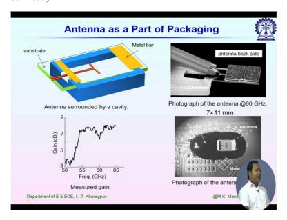
This is the zoom in view of the structure of the fol um sorry these are dipole antenna with similar structure guard ring and right hand side it shows the photograph of the fabricated structure and look at the gain. Previously we are getting typical gain value below 0 DB. Now with all this precautions when we could avoid coupling between the radiator and the MMIC structure not only that power coupled to substrate.
