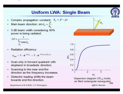
Let us continue with the uniform leaky wave antenna. This is a typical example here it shown for rectangular wave guide we are measuring the beam direction from broad side direction its given by theta M as we discussed the propagation constant its complex here. It can be written as beta minus J alpha then main beam direction it is being determine by beta.
