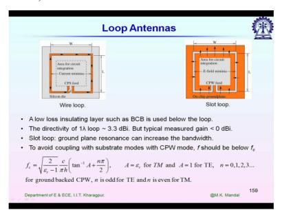
We are having 1 wire loop antenna and its length is 1 lambda at the operating frequency and typical gain we get from 1 lambda loop is more than 3 DBI but when we fabricate it on silicon because of those increased losses realised in always less than 0 DB we will be having some negative value. In this particular example this loop is being fabricated on DCB material which is placed on that silicon.
