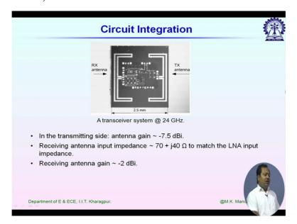
So now we know how to choose the type or radiator so next how to integrate them inside chip because in chip we also have circuit. So we if we use any metallisation for the circuit implementation obviously there will be coupling between that metallisation used in circuit and the radiator. Thats why radiator it should be placed as far as possible from the circuit board.
