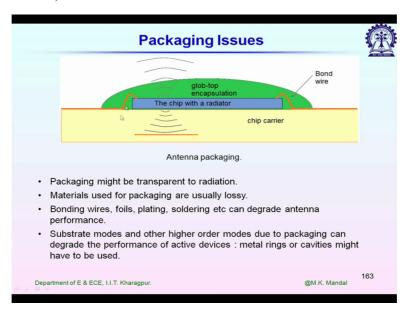
Next packaging issues, in practice always we will be using some sort of packaging material to protect the chip from different weather condition it showing a scenario like that a glob top encapsulation is being used as the packaging material. Then whatever material we use for packaging it is usually lossy material.
