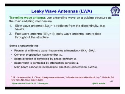
So thats all on on chip antennas, next topic we are going to start as leaky wave antenna. So till now whatever we have discussed we are using some sort of resonator structure and its length is typically lambda g by 2 or lambda g at the operating frequency now we will see some of the antenna another group of antennas where the antenna length is much more compare to lambda g.
