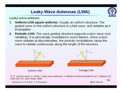
We will discuss now 1 by 1. Now under leaky wave antennas we have again 2 different categories we have we may have uniform leaky wave antenna and we have periodic leaky wave antennas. Here are the examples shown here. You can see a rectangular wave guide where 1 longitudinal slot is placed on top of the on the top wall and it is 1 example of uniform leaky wave antenna it usually radiates along the length.
