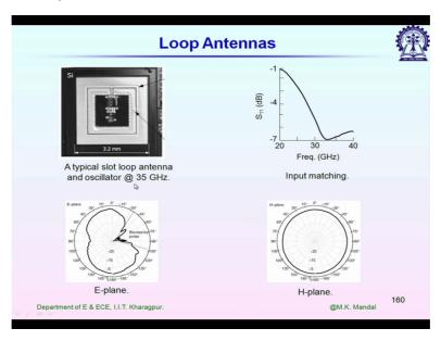
These are fabrication example from IBM. It is design for 35 gigahertz application and typical dimension it is shown left to right is 3.2 millimetre and you can identify the antenna structure we have a slot loop feed by the CPW line and also we have a ground plane and look at the S11 plot. Its bandwidth is quiet high the matching bandwidth.
