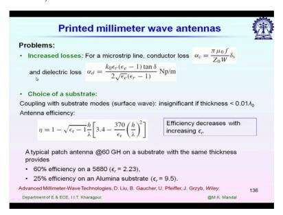
So first one already we know at millimetre wave frequency for example for a micro strip line conductor loss is given by this which we already learnt at it increases with frequency. Dielectric loss it is also a function of frequency it also increases at millimetre wave frequencies. Next important point comes choice of a substrate. What should be the dielectric constant of the substrate? What should be the tan delta of the substrate?
