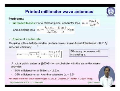
What are the problems we faced at millimetre wave frequency? At millimetre wave frequency if we want to design any antenna on printed circuit board or laminates. Then the losses what are the sources of losses already we know. And this loss increases with frequency. So do you remember the 3 sources of losses? The first one is dielectric loss, second one conductor loss. And third one loss due to surface wave generation.
