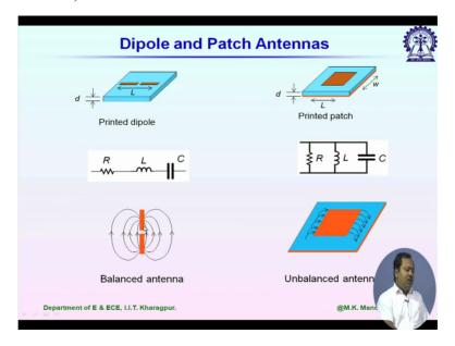
Now if I look at the electric field plot of any resonating dipole antenna it looks like this. So the length of this antenna is lambda g by 2 at resonating frequencies and if you look at the electric field it is maximum on the central plane. And we have in the far field radiation electric field is parallel to the wire or this line of this dipole antenna.
