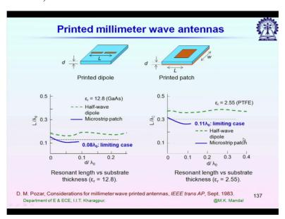
Next we will see resonating length of the antenna its a function of frequency not only that it also depends on epsilon R of the substrate. Why? Because of this fencing field component for different epsilon R we will be having different fencing field components so we have different length correction factor because of that. So we will take a brake then we will start again. Thank you!
