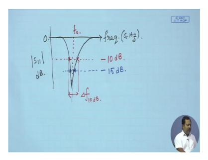
If I plot frequency let us say in gigahertz versus S11 which is in decibel scale if S11 in DB is 0 DB that means whatever power I am feeding to antenna it is being reflected back 100 percent power is being reflected back to source. Now if the antenna accepts power then we have some negative value of S11 so let us say we have measured the S11 or we have simulated the antenna structure from that we have knowledge on S11 and when we plot it.
