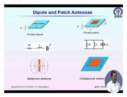
So now look at this electric field plot we have fencing field. Left hand side and right hand side so it represents the length of this antenna in this direction now this length it should be lambda g by 2 at the resonating frequency. And we will be having maximum radiation intensity in the broad side direction of this antenna.
