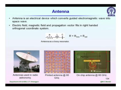
So if I look at the different antennas already available or are being used at millimetre wave frequencies first category it shows a parabolic reflector antenna. So where we use 1 feeding antenna we call it feeder. It can be horn antenna or anything else and then the electromagnetic wave is reflected by this parabolic reflector so we use this for astronomy application where we need extremely high gain and very narrow beamwidth of the antenna.
