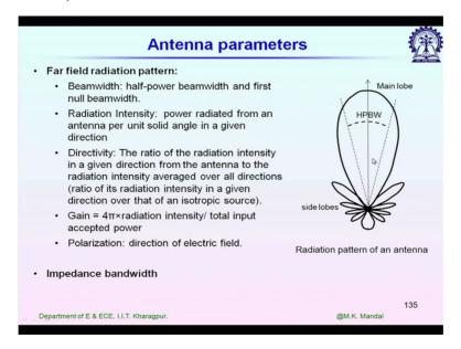
Now for a general antenna structure we have to deal with many parameters so how we define the characteristics of an antenna? There are several parameters we should know the parameters first. So for example the first important parameter is far field radiation pattern. So what we do? We just measure the electric field or power which is square of electric field.
