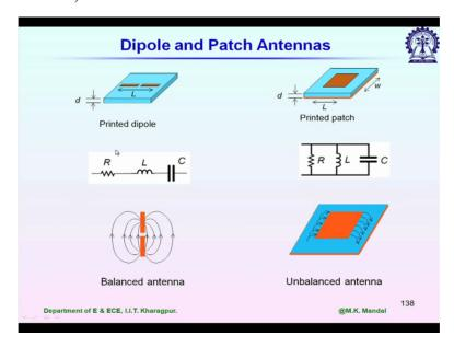
So if you look at this equivalent circuit for printed dipole and printed patch both are resonating antennas but in the equivalent circuit printed dipole is represented by a series resonator. Where this capital R it includes both the radiation resistance and the loss in the antenna structure itself. Whereas for the printed patch its a parallel resonator and R represents same things.
