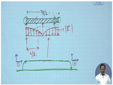
Let me start from a very basic resonator let us say we have a micro strip line resonator of length lambda g by 2. Obviously at the resonance frequency now both of this 2 ends they are open circuited so at resonance frequency if I plot electric field along the line then we will be having maximum left most and right most edges. And if I plot current distribution so this is the plot of electric field.
