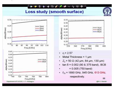
Because at millimetre wave frequencies it creates the main problem in any MMIC. So let us see more studies. So these we are we have calculated these losses by using full wave simulator. So we are considering 3 different thickness of substrates 15 micro meter thickness, 30 micro meter thickness and 45 micro meter thickness of BCB substrate. It is popular at millimetre wave frequencies or even at terahertz frequencies and typical tan delta value for 100 gigahertz and 400 gigahertz is point 002.
