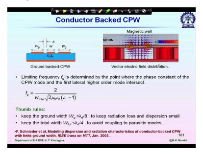
Let us start CPW line Coplanar waveguide. It cames in 1960s. Let me draw a coplanar line first. How it looks?
