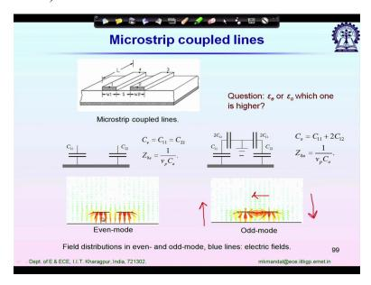
So for even mode since epsilon E is higher small length will show more beta so if I consider let us say a fixed length of 5 millimetre microstrip line For left hand side case and right hand side case so for left hand side if the 5 millimetre length it represents some electrical length equivalent electrical length let us say 180 degree at some given frequency.
