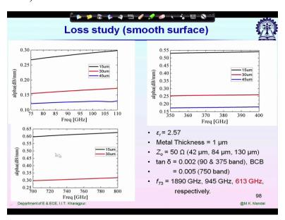
So if I go back here, you can see we are plotting it only for 15 micrometer and 30 micrometer and that 45 micrometer is absent here. Why? Because for 45 micrometer will be facing that transverse resonance phenomenon. Because already we have calculated FT3 is 613 gigahertz for the third case.
