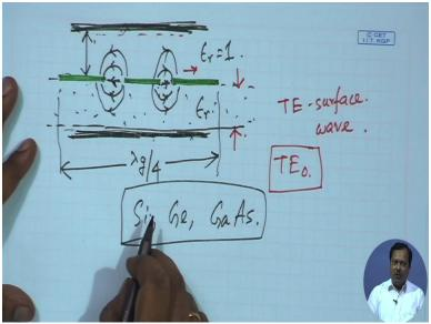
So we have a central conductor which is a central strip and its separated by from 2 ground strips and together they sits on a dielectric layer. You can consider it as a couple slots. This is the cross sectional view. So inside we have electric field if you remember that odd mode and even mode excitation so we prefer even mode excitation so that this 2 extreme ground they will be at same potential and in that case the electric field configuration will be like this.
