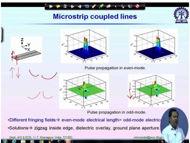
Let me show you the time domain propagation so you can see the strips and in these figure we are showing the propagation direction is Y and we are placing 2 mi millimetre wave sources at these edge left hand side. So here right here so let us first consider the even mode excitation that means these 2 sources they are in same phase.
