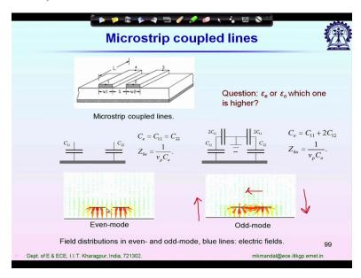
For the even mode case we don't have any electric field from left strip to right strip. So if I consider a mid plane which is perpendicular to this and it is placed just in between these 2 strips then no electric field is passing through that plane. Not only that the electric field left hand side and right hand side it becomes parallel. So we can call this plane a PMC or open circuit condition.
