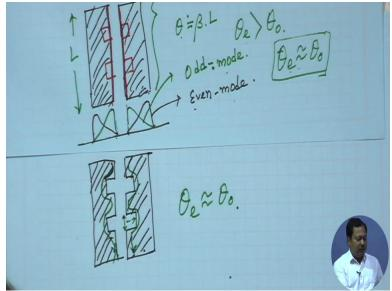
Let us say we have a coupled line system. I am drawing the top view so this is the left strip and this is the right strip. Now if I plot the surface density of surface current component on left strip and right strip for even mode and odd mode they will have different variation. So in even mode this current will be more concentrated on outer edge so this is for the even mode scenario and in odd mode we have some sort of attractive effect.
