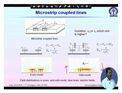
And for this one then this coupling it might be through magnetic field so for even mode we called it magnetic coupling. And right side we can see it clearly we have electric field from right strip to left strip so the coupling is due to electric field and we call it electric coupling.
