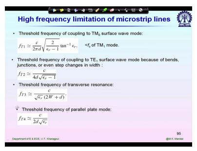
This is the threshold frequency of transverse resonance and we are considering it for that given 50 ohm line in the substrate.
