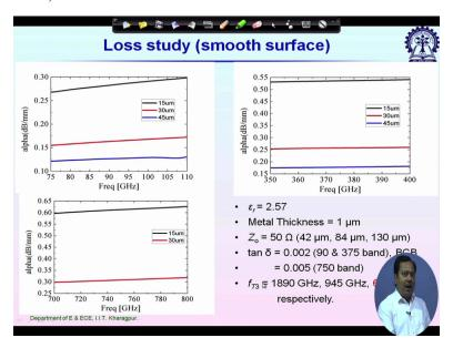
So FT3 it is minimum among all these four for each and every case for the first substrate its coming 1890 gigahertz. For the second substrate it is 945 gigahertz. And for the third substrate with the thickness 45 micrometer since it is having the widest line it is having the minimum FT3. So the third substrate we cannot use let us say about 600 Gigahertz.
