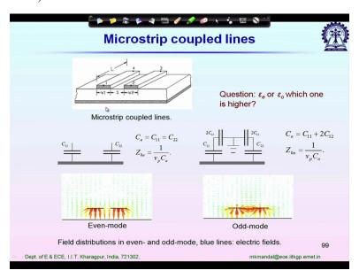
So let us see what is that. We have two coupled microstrip line. We can excite this coupled microstrip line by using 2 RF signals in 1 case it can be in same phase and in the second case it is in opposite phase 180 degree phase difference between these 2 signals. So the first cases when the 2 signals are in same phase we call it even mode condition. And the second case we call odd mode condition.
