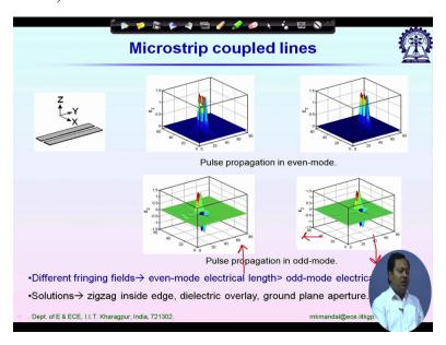
Because if I look at this plot the outer tips are higher compare to the inner tips so there is coupling effect.
