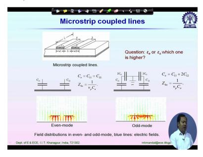
In even mode condition, when we are exciting by the source having same phase component the electric field this is the plot of electric field on a cross sectional plane. You can see the black colours microstrips and this black colour line it represents the ground. So the direction of electric field in same direction and there won't be any coupling between these 2 strips.
