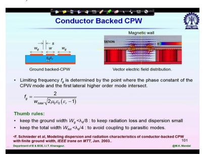
So you can identify the top layer CPW line. W this is shown as the width of the signal line. WG this is the width of the ground and we have 1 additional metal layer. It is the ground plane of the CPW line. And now you see at least in 1 side we can directly place our packaging wall and on top of this of course again we have to maintain some minimum separation. So we will take a short break. Then we will discuss on the ground back CPW line. Thank you.
