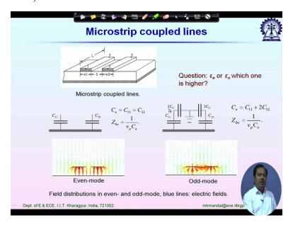
Let us consider a special scenario. Microstrip coupled line. We use microstrip coupled line whenever we go for component design components like couplers, filters and we deal with even mode and odd mode analysis of coupled lines.
