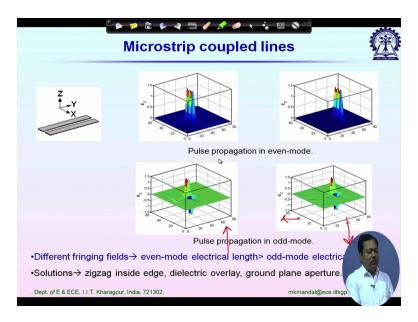
So in odd mode excitation you can see in 1 case, this for the left strip the electric field below strip its in this direction and for the right strip it is in bottom direction and not only that we have electric field coupling between these 2 strips. For this figure it shows that electric field right to left strip.
