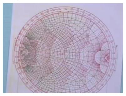
What is the center of the circle we are calling C with the subscript F to show that for a given noise figure this value is this center is this and radius is this. So obviously here if F = Fmin you can check that If F = Fmin let us see the N value so where is N so if F is Fmin N becomes 0. So
