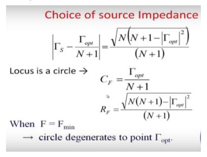
Which is equal to then gamma source resistance just equals the gamma opt obviously that is also the definition of gamma opt so circle degenerates to point that part is easy. That means if we always design for Fmin we get it but sometimes we do not because if so much noise stringent noise figure is not require then we try to design for a bit higher noise figure which will serve our purpose but that will give us some more gain because we know gain in also important.
