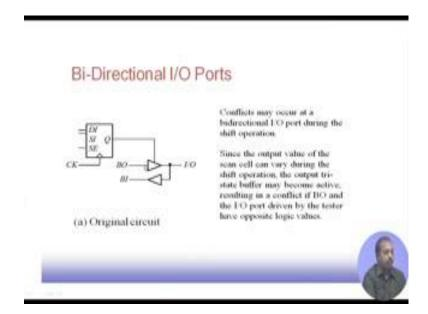
Then there are bidirectional I O ports like say this is a see a structure where we have got this from an input output pin; bidirectional pin there are buffers. So, this buffer is going for putting the value to the buffered input, similarly the buffered output will go through this buffer and it will come to the output.
