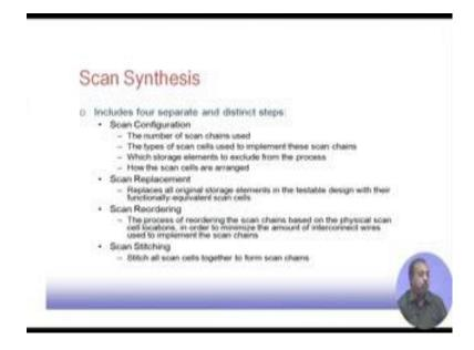
Then comes scan synthesis, the first part of this scan synthesis is scan configuration. So, this will be the first input that we have is the number of scan chains used. So, if I have got a single chain then what will happen is that all the flip flops that I have. So, they will
