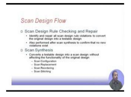
We will see; we will look into this design flow. So, first part of this design flow is the scan design rule checking and repair. So, this is for identifying and repairing all scan design rule violations to convert the original design into a testable design. So, whatever design rules we have seen, the scan design rules we have seen; so they are checked and if there is a violation then they are corrected for making the design test table and it is
