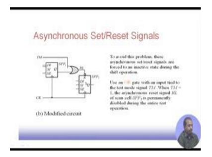
And for doing this thing, again the way we have to do it is that this in under the test mode this TM line; this R L is put through an OR gates so this Q output and this TM so they will be odd here and then it will go to this thing.
