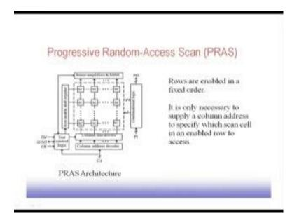
So, rows are enabled in a. So, the sense amplifiers are there. So, basically this column driver and sense amplifiers are there. So, they will drive individual column and sense amplifier will since the difference between SD and SD bar line and see the difference. So, rows will be enabled in a fixed order. So, that we can read all these scan cell elements and it is only necessary to supply column address to specify which scan cell in
