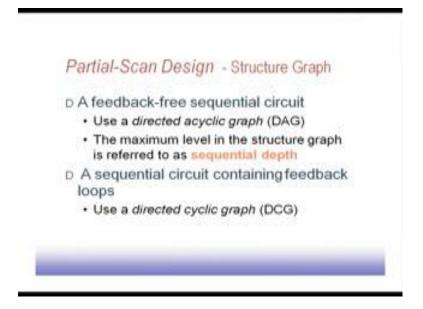
So, this structure graph, so if feedback free sequential circuit. So, that is what we are looking for the, for that purpose we use it, first of all we construct a directed acyclic graph. The maximum level in the structure graph is referred to the sequential depth. I think there is an example.
