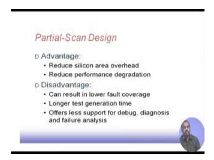
Why partial scan design? So, it has got advantages like the silicon area overhead is less because least number of flip flops are converted into scan flip flop. And performance degradation is also less because for flip flops. So, we are not putting any multiplexer before them. So, as a result, if some flip flop is on the critical path. So, they are at performance is not affected.
