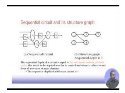
So, here you see that, suppose this is a sequential circuits. So, where we have got this flip flops F F 1, F F 2 feeding this combinational logic C 1. Similarly, this C 2 is feed by F F 1 and F F 2, C 1 is generating output for F F 3. So, this way it is occurring.
