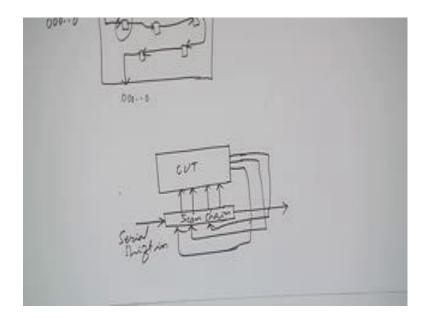
Now, we have made a shift register which is also known as scan chain. So, in this scan chain we serially shift in. So, this is the serial shift in and after we have got this data shifted in. So, we load this pattern. So, this pattern will be applied to the circuit by means of applying in the capture cycle by applying this input to the circuit. So, the test pattern is applied.
