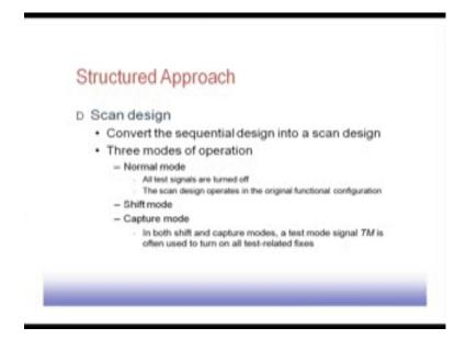
Next we will look into the structured approach for this DFT design. So, this they come under the broad heading of scan design. So, it says it converts the sequential design into a scan design and as we have notated earlier, in scan design what happens is that? This flip flops that we have in the design. So, all those flip flops are converted into scan flip flops and they are connected over a chain.
