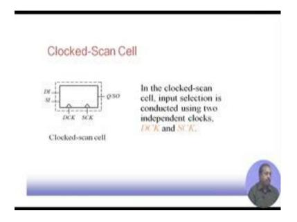
So, this is another possibility. So, the cell is designed in such a fashion that it operates with two different clocks; so this when, the data clock is given, so the circuit operates in a normal mode and when this scan clock is given the circuit operates in a scan mode.
