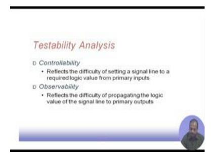
So, all these testability analysis technique so they try to measure two values; one is called controllability, another is called observability. So, controllability it reflects the difficulty of setting a signal line to a required logic value from primary input. So, what happens is that if I have got some circuit, then if I want to say put this particular line on to some logic value.
