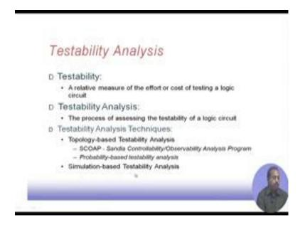
We will start with testability analysis. So, testability is a relative measure of the effort or cost of testing a logic circuit. So, how much effort we are putting, we need to put for testing logic circuits. So, testability analysis is process of accessing testability. So, there are various ways by which we can do this testability analysis; one is known as SCOAP approach which is Sandia controllability observability analysis program; there is another
