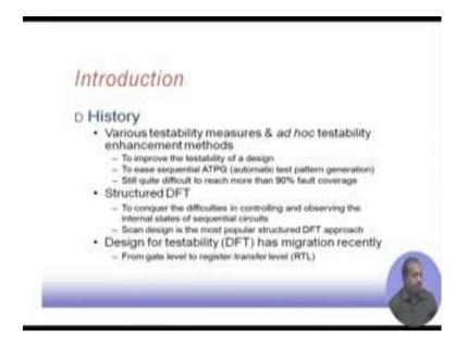
There are various testability measures and ad hoc test ability enhancement methods that have been used. So, for let we improve the testability of a design. As I said that for a design it maybe to complex, so we cannot access one particular line from primary input, we add a multiplexer and put it somewhere so that the line becomes controllable.
