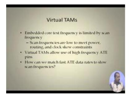
So, the first one in that category is known as virtual TAM. So, virtual test access mechanism. As the name virtual means that the actually the TAM lines are not more, but it gives an illusion that the TAM lines have been increased.
