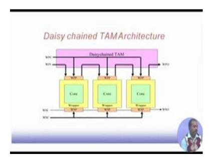
But here in this case once a test is going on, so nobody else can be tested, so that is the problem with these daisy-chained structures.
