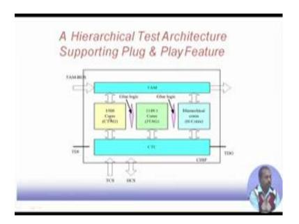
Next one is hierarchical test architecture. So, this is basically, so this is a typical situation. We have got these cores supporting this 1500 series. So, they are called c tag cores, because they are supporting this core interfacing. So, they can be directly connected to this they can be they can have both serial connection as well as parallel connection. So, they can be connected through this TDI line serially or they can be connected with a TAM-BUS. So, I have both of them can be used.
