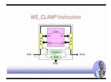
So, then there is a parallel preload WP preload operation, so this is again the same thing that WSI will be put into the bypass mode. So, this wrapper serial input is not going to affect this WBR, so that is going into bypass mode. And whatever has been loaded into this WBR, so they are available as preloaded state. So, similarly this WBR content is also available as a preloaded state so whatever values were preloaded, so they are available at the output of those parallel outputs.
