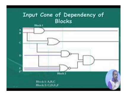
So, the cone of dependency as we were telling that if this is block one then the cone of dependency has got inputs A, B and C; similarly if this is a block 2, so cone of influence is the pattern are the input, so D, E and F.
