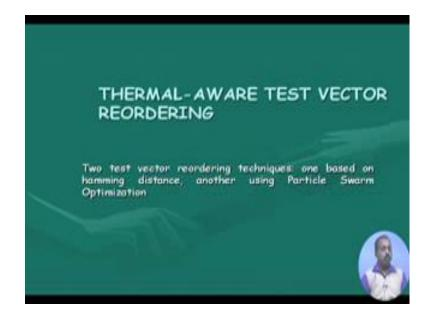
So, a very basic strategy that can be followed is the test vector reordering. So, we have seen that the test victor reordering it can reduce the test power, so similarly this test vector reordering can also reduce the temperature. So, we will see some techniques based on some techniques based on hamming distance and another technique based on a more detailed approach which is known as particle swarm optimization.
