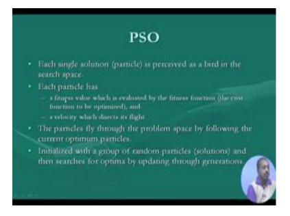
So, each single solution or particle is perceived as a bird in the search space. Each particle it will have a fitness value, which is evaluated by the fitness function, the cost function to be optimized and a velocity which directs its flight. So, there is a fitness every
