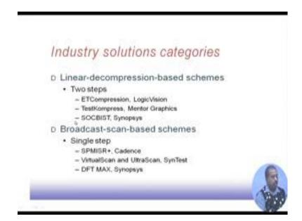
Now, this linear decompression based schemes. So, there are some schemes which are based on linear decompression. So, these are the schemes like ETCompression,
