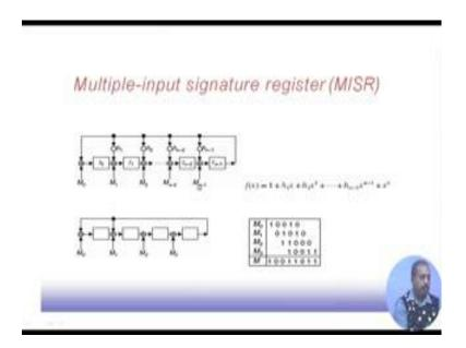
So, if this is one multiple input signature register. So, we have got this r 0, r 1 up to r n minus 1. So, this is represented by this characteristic polynomial 1 plus h 1 x plus h 2 X square h n minus 1 x n minus 1 plus x to the power n. So, depending upon the values of this h s, this characteristic polynomial is getting defined.
