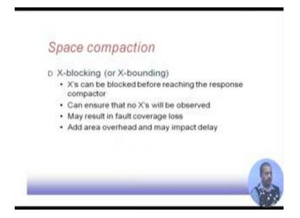
Another possibility is space compaction is known as X-blocking or X-bounding. So, Xs can be blocked before reaching the response compactor. So, we can say that if there is some unknown value coming. So, we can block that value. So, we can ensure that the Xs
