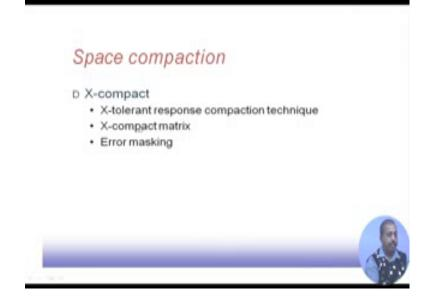
So, next we will look into this space compaction techniques, first one in that category is the X-compact. So, this is X-tolerant response compaction technique. So, what happens is that it will tolerate the excess that the unknowns that come in the response. So, it will tolerate that. So, will have a matrix which is called X-compact matrix and then this error masking will be utilized.
