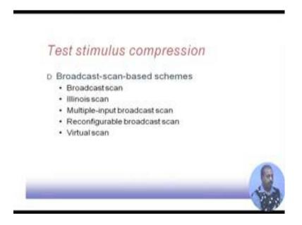
So, that way it is going to be helpful. Next we look in to a test stimulus compression in that category; we will be looking into broadcast scan based scheme. So, broadcast scan based scheme means that there are multiple scan chain, and these multiples scan chain are fed simultaneously in a broadcast mode, and there are several such scan mechanism so we will look into some of them.
