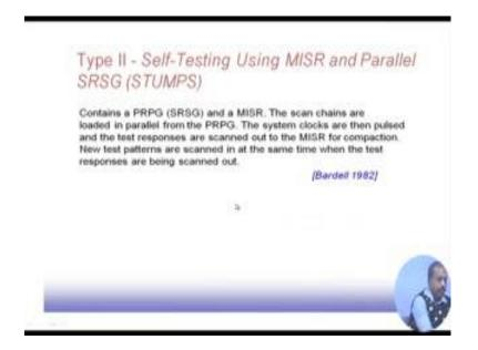
Then there is another very popular structure which is known as self testing using MISR and parallel shift register, SRSG. So, they are called that is called stumps. So, this contains a pseudo-random pattern generator and one MISR the scan chains are loaded in parallel from the pseudo-random pattern generator the system clocks are then pulsed and the test responses are scanned out to the MISR for compaction. So, let us see how this structure looks like.
