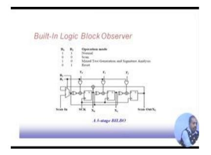
So, this is a typical BILBO structure you see that is has got several modes. So, there are 2 control signals B 1 and B 2 and this functional data when B 1 equal to 1 and B 2 equal to 1 what is happening is that Y 0 value is getting loaded into this clock. Similarly Y 1 value is getting loaded into this flip flop, Y 2 value is getting loaded into this flip flop. So, that way for both of them being equal to 1, this circuit operates in the normal mode Y 0, Y 1, Y 2 loaded into this latches.
