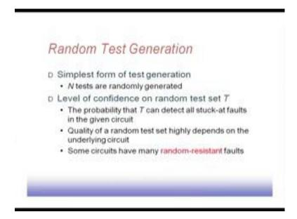
Random test generation, this is the simplest form of test generation. So, we generate N randomly, generate N random test pattern. So, this random test pattern, basically it say if it say 2 valid circuit, 2 valued logic, we apply random 0 1 patterns to the inputs then see if whether what type of output it produces.
