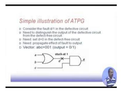
Let us take a start with the simple example. So, consider a fault which is a D stuck at 1, we want to, this is the circuit we having 3 inputs a, b, c and 1 output e and we want to
