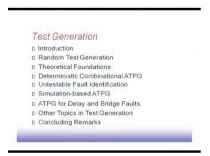
Random test generation means we randomly apply some test patterns and see whether some faults are getting covered or not and it is interesting to note that a good number of faults are detected by some random patterns and it is many times it is up to 70 to 75 percent faults of a circuit that are detected by random patterns. So, the remaining faults,
