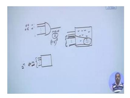
For checking that 8 input AND gate, output stuck at 0 stuck at 0. So, this lines stuck at 0. So, I need to push a 1 at this point, now to push a 1 at this point, I must be able to apply all ones at the input.
