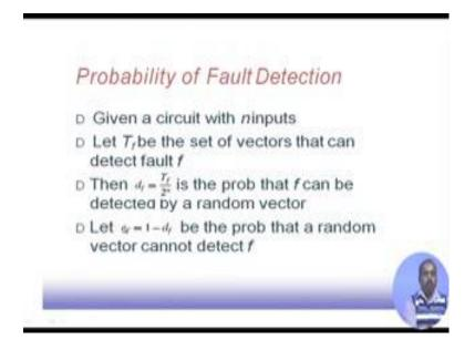
Probability of fault detection, given a circuit suppose which have a n inputs, if T f be the set of vectors that can detect fault f then d f is T f of 2 power n it is the probability that f
