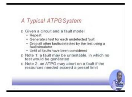
A typical ATPG system will work like this given a circuit and a fault model, what it will do? It will repeat the following steps what generated test for each undetected fault. So, initially all the faults in the circuit are undetected. So, it can try; it can try to generate a test pattern for that. So, if it successfully generates one test pattern, certain faults in that
