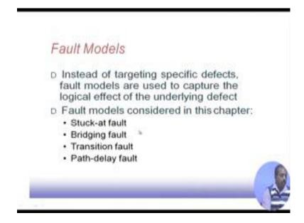
As we have already seen that physical defects are not handled directly rather we have some fault models and with respect to that fault model, we need to generate that test pattern set. So, fault models that will be considering in this part of our lecture as stuck at fault bridging fault default transition fault and path delay fault. So, these are the types of faults that will be covering in this part of the lecture.
