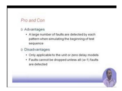
Several faults are getting simulated parallelly, advantages we have got a large number of faults that are detected by each patterns when simulating the beginning of the test sequence. So, as a result what will happen is that since we every simulations since it is handling a number of faults instead of single fault in case of serial simulation or series fault simulation.
