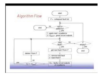
This is the flow of the algorithm. So, start with the then we start with the collapsed fault list. So, new w patterns, as soon as you get a new w patterns from the test set. So, we apply the next w patterns and output good is the good circuit output.
