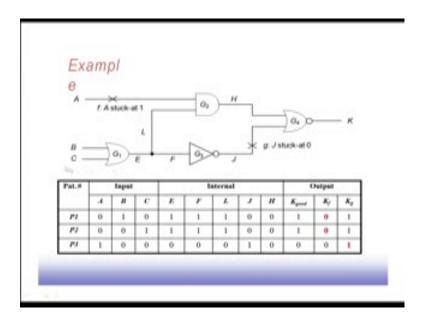
We want to see that whether we are; we can get this thing that is f stuck at 1 and G stuck at 0. So, these 2 faults, primary input pattern, we have got 3 patterns, P 1, P 2 and P 3 and for then this A, B, C value this is P 1 is 0, 1, 0, P 2 is 0, 0, 1 and P 3 is 1, 0, 0. So, for first one is the; for the good circuit what is the response? So, we simulate this circuit for in the absence of all these faults F and G and we see that this K good is 1, 1 and 0 for the 3 pattern.
