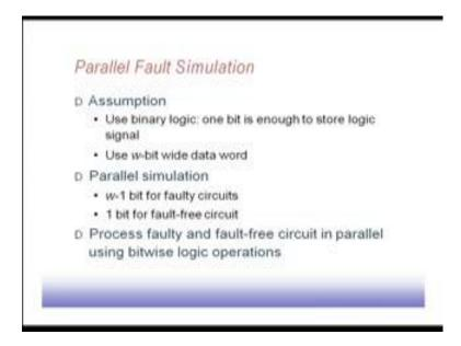
First one is the parallel fault simulation, it is assumed that we use binary logic that is one bit is enough to store logic signal. So, we are not looking into ternary or this higher order logics, but only binary logic.
