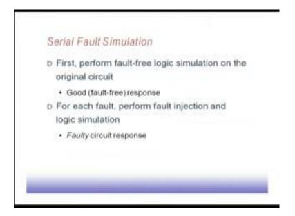
The most simple fault simulation technique is the serial fault simulation. So, what we do in this case we first perform a fault free logic simulation on the original circuits. So, we have got the test pattern set for the test pattern set we want to determine, what are the fault free responses from the circuit? So, these are called good or fault free response.
