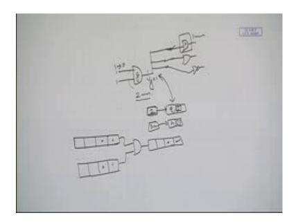
Now, for every single line that we have, we have got this particular word available, now suppose this is 1 AND gate. So, it has got 2 input and with both the inputs we put these 4 bits, similarly at the output also we have got this 4 bit space. So, the idea is that if the first bit will be computing and of this and this. So, if these 2 are ended, the results will be stored here.
