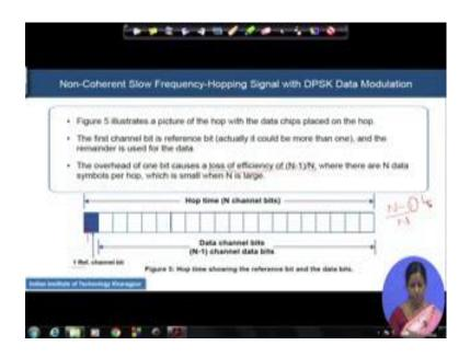
So, this is the figure that illustrates how we pack the signal before transmitting. So, these are the all the DPSK data bits, that will be transmitted and remember for DSSS system, synchronization is a very typical issue, for that we usually sent 1 or 2 reference channel bits, to identify to estimate the frequency or change the timing set in the DSSS system, and then we try to relying the risk part of the frame bits, so that we can really extract our data.
