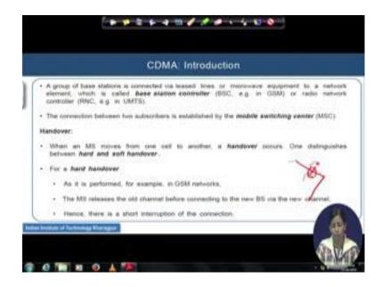
This hard handover as I was talking about; that hard handover is performed in the GSM networks the weight is done is, the whenever the mobile station is a reaches at the boundary of a any cell: suppose this is the boundary of the cell and mobile station is crossing the boundary he just leaves one channel and he is just joints the channel of which corresponds to the next cell and the base station it can be sub by the next base station.
