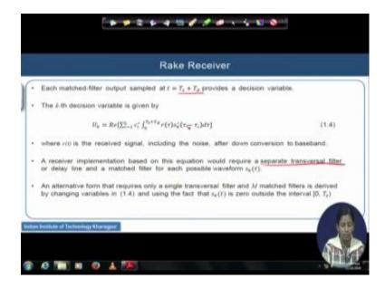
So, now the each matched filter output now you have to sample, the sampling should be done at the gap of the symbol duration plus T d, it is not T plus t d it should be T s plus T
