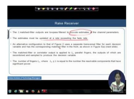
So, now that capital L matched filter outputs are low pass filtered and then it is providing us the estimate of the channel parameters. This estimates we should update at the rate of which should not exceed the fade rate. So, it should be actually at per the rate of the fading and the rate of the slow or fast fading I mean, so that estimation should be according to the rate at which the channel is changing.
