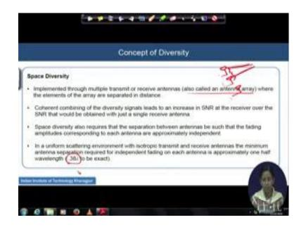
In the space diversity, we implement the multiple transmit or the receiving antennas, we called them the antenna array, I draw it in the last slide, where this elements and the arrays are will be separated by a distance. The coherent combination of all these array elements I mean this signal received from these array elements, we will be actually in help us to increase the signal-to-noise ratio compared to a reception via single received antenna.
