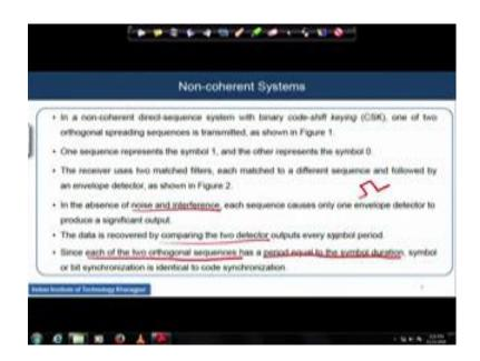
This is the structure of the transmitter. Let us see how the receive values looks like, the CSK so; I will give more information let with respect to the transmitted figure. Remember that in absence of this noise and the interference each sequence will cause only one envelope detector that actually in the figure 2, let us go and come back because otherwise it will be hard to understand some more points that is explained in this typical slide.
