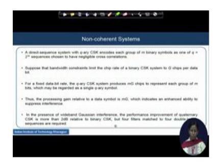
And now the another extension of this understanding with q-ary CSK encoders, that from each group of m binary symbols as one of the q equal to 2 to the power n sequences it will be chosen, and that sequence should have a very negligible cross correlation values for q-ary CSK transmission,
