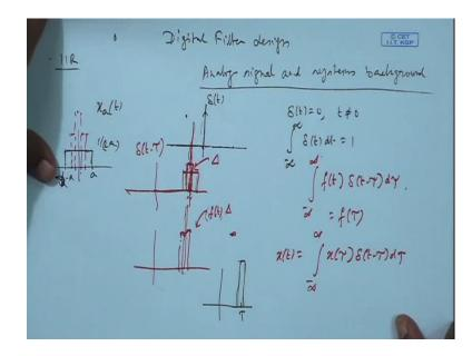
Now, we will be going for filter design, which is a very complicated not complicated, but because lot of insight and we need analogs signal processing background. We will take a quick review. So, we will now go for the digital filter design, IIR filter design for this. We require analog signal and systems background.
