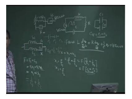
Similarly, if the two springs connected in parallel, this is the one spring and this is another spring connected in parallel. This is S 1; this is S 2; force is applied F. Then what
