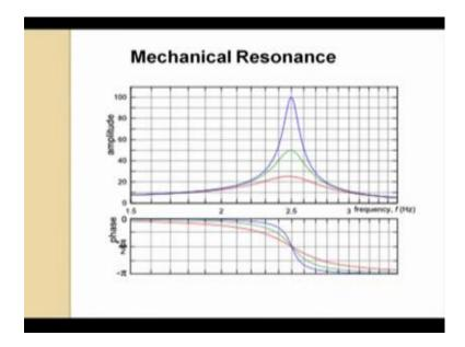
Now, if you see, if I draw, so I said the mechanical resonance maximum power transfer will be happen at omega equal to omega 0. Now, if I draw the curve maximum power transfer curve, if you see the curve in the power point, what is saying that if I take axis this axis is omega and this axis is the power.
