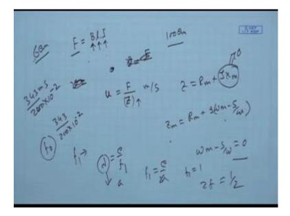
So, force produced by the loudspeaker F mechanical force is nothing but B into l into I, magnetic flux B is the strength of the magnetic spill, l is the length of the wire, I is the current pass through the wire plus density air gap force acting on a voice call effective
