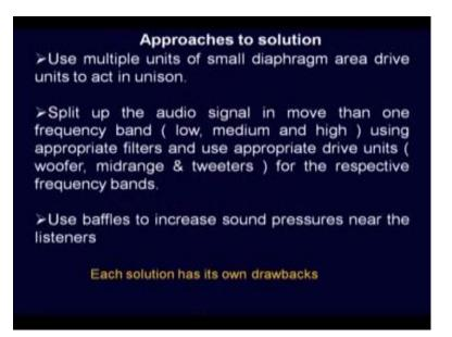
So, large acoustical energy when I want then if I want a large diaphragm maybe the high frequency component or frequency response of the loudspeaker maybe dropped or high frequency component maybe cut out. So, what is the solution, solution is that use multiple unit of small diaphragm. So, I want to increase the acoustic power.
