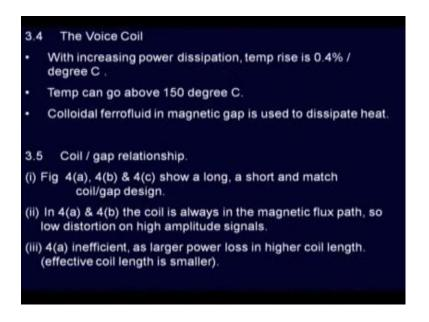
Then the voice coil. What is the voice coil with increase the power dissipation temperature will be rise then temperature can go up to 150 degree centigrade. So, how do reduce that things loss by coil gap the coil gap relationship.
