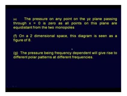
So, if you see the dipole radiation pattern this is the figure of merit of figure of eight for the dipole, I am not reading the slides. Now, I come for so you know what is monopole and what is dipole what is source strength. (Refer Slide Time: 12:53)
