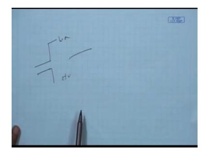
So, for the high frequency, I can divide at the input signal in two paths - two area one is the low frequency and another one is the high frequency then I can drive the two loudspeaker. So, signal has to be split tweeter is the high frequency and that other one is the low frequency.
