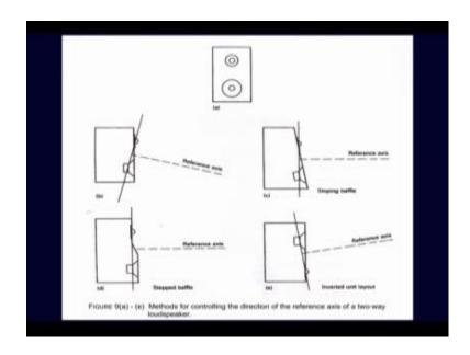
Then I show you something on reference axis loudspeaker housing is not that easy. So, if it is this tweeter and main loudspeaker in this the same plane then the same reference axis is this one. If it is housing like this then the reference axis is this one. So, radiation power will be in this direction and this reference axis is this if I put like this to cope this is the way reference axis is this. So, different construction gives you the different reference axis.
