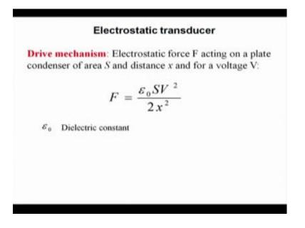
Similarly, another kind of example is that electrostatic transducer where I use capacitance - variable capacitance as a transducer.
