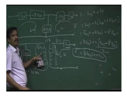
So, the equivalent electrical circuits, let us I draw in cleanly it will be V, there will be a Z E B, there will be negative impedance minus phi Z E B, then there will be a here minus phi Z E B, Z m o and terminal here I put on impedance phi Z E B. Then I apply a voltage here V, current I will be flowing, and I apply a force here F, particle velocity u will be flowing equivalent electrical circuits.
