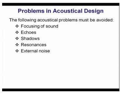
Then what is the problem in acoustics design that is the few problems in acoustical design we have to avoid focusing of sound when I design auditorium there should not be any particular place where the sound is focused. We have to have avoid echoes there should not be any echoes we have to have avoid shadow what is sound shadow we discussed diffuser in diffraction if there is a obstacle of the sound it create a sound diffraction.
