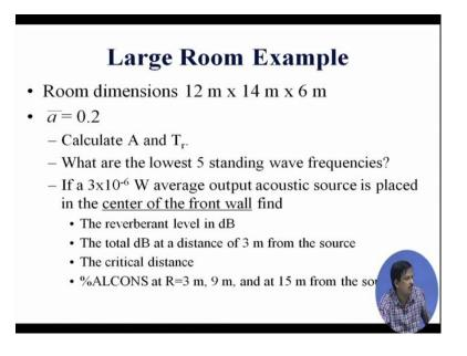
Now, for the example, let us do mathematics that suppose I given the room dimension is given 12, 14 and 6 meters, this is a squared kind of room. And there A is given average acoustic is given, calculate capital A in Sabin and T r means reverberation time, can you calculate T r.
