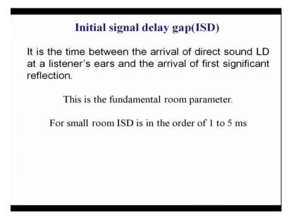
Lets two speaker I place in the two side of the wall of the front of the auditorium by stage side of the auditorium then from speaker to any distance I can calculate the percentage ALCONS speech intelligibility then the another term is called initial signal delay gap. So, I said then if in any enclosure room if I hope if I play a sound source then at any point of from the source it will be direct sound and there will be a reflection sound.
