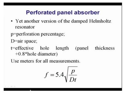
So, absorption there is some absorptive material also required. So, what kind of material is there for absorption I required a slot absorber I can use a slot absorber, you can read the slide for that use of the slot absorber or I can use the perforated panel absorber where the frequency is formula is given.
