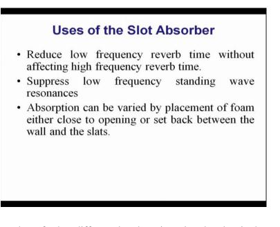
So, there is a number of other diffuser also there is a slot absorber is there that use slot absorber to reduce the slot absorber. So, there is a diffuser. Now there is a absorber also what I said I have to make the I have to make the auditorium such that there is a no focusing of sound that is the job of the diffuser. So, all the reflective surface must be treated as a diffusive reflection no poly surface if it is poly surface regular reflection which has to be avoided.
