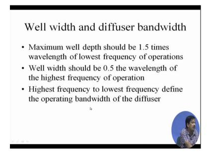
Then there will be a well width and diffuser bandwidth. So, if you see there is a slot like this way, wall then we have a slot, slot diffuser you put a slot.
