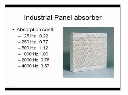
So, perforated panel absorber like this; this is an absorber acoustics absorber. So, absorption coefficient is given for different frequency. So, while you buy a absorber from the market or acoustic styles from the market the absorption coefficient with the
