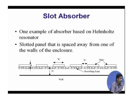
If you see the auditorium the front part to just enclosure to the stage this curves to the stage there is a slot wooden slot, slot is placed on the wall. So, this slot width and depth is not random it has to be a designed best on that requirement. So, you know the frequency of the operation of the auditorium then we have to design the depth on based on that equation.
