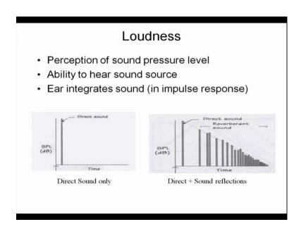
So, I can say this is the direct sound; this point the sound is created or the sound pressure level will be developing based on the direct sound. So, direct sound will come here with
