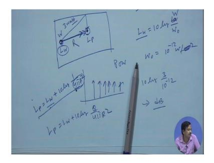
So, suppose I have an auditorium, let us draw it, and let us this is. So, I have sound source here; in here I want to calculate the power sound intensity or sound level, sound pressure level. Then since it is a semi reverberant room, there is a direct sound and there will be a reflected sound. Then the reflected sound will be there. Note most of the real auditorium in practical purpose is semi reverberant room.
