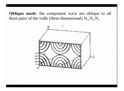
Then there is a call oblique mode. The component wave are oblique to all three pair of the surface that is x, y, z -3 I N x, N y and N z three nodes are exist, so that is f 1 1 1 first node, f 1 1 2 may be f 2 1 1. So, all kinds of combination will be possible, first harmonic second harmonic third harmonic, all combination will be possible that is called oblique mode. If it is tangential mode, only two will be there x and 1 0 1 or f 1 1 0 all are tangential mode will be there.
