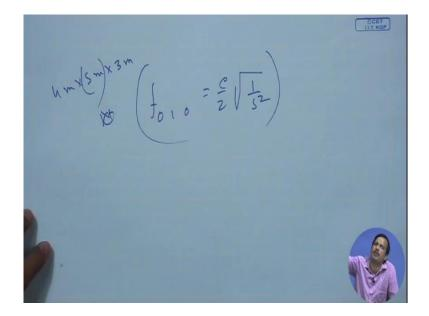
Lets I give an example for that node calculation. I told you that suppose I have a small room; room dimension is 4 meter, 5 meter and 3 meter. And calculate the first node lowest axial-mode lowest axial-mode. So, you can say f in any axis which is lowest when which will be lowest when the denominator is high. So, it is can be 0 1 0. So, it is it is c by 2 root over of 1 by 5 square lowest axial node frequency is this. Then I can all other
