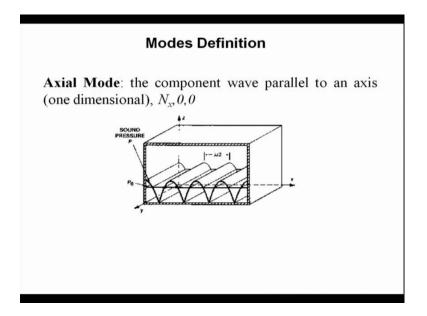
So, mode definition, now I came to the mode definition. Axial mode the component wave parallel to an axis is in one dimension. So, suppose in this room the node is created parallel to the axis only the horizontal the surface ground surface the node is created. So, only the node is created along the x, y plane only. So, all are you can say it is created alone the x-axis only standing node, so that is why it is called axial mode or it may be.
