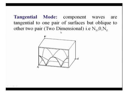
Then there may be a tangential mode. The component waves are tangential mode to one pair of surfaces but oblique to other two pair that is called two-dimensional. So, see that it is parallel to one pair of surface, but oblique to other pair so; that means, it should here two nodes. So, it is  $N \times N$ ,  $N \times N$  or you can  $N \times N$  or you
