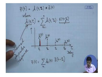
So, we could write these expressions in a better way and state that we have r tilde t is equal to filtering of s tilde t with h t of n, which we have as h t comma tau n convolved with s tilde t. Where, we could write h t comma tau is equal to the sequence n equals 1 to capital N h of t comma tau n is called convolution of h t comma tau times delta tau minus tau n.
