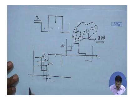
Suppose, I have a signal sequence which goes like this, so at the receiver at this instant of time what do I accept; what I accept is the signal which was transmitted here gets scaled by h 1 plus the signals which was transmitted here gets scaled by h 2 plus what was transmitted here gets scaled by h 3 and so on and finally we sit over here.
