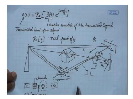
So, what we will do is we will write S of t as the transmitted band pass signal is equal to the real path of S tilde t which is the complex envelope of the transmitted signal - e the power of j 2 pi f c t where this is the complex envelope of the bypass of the transmitted signal.
