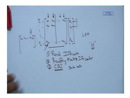
We were saying that there is w 1 which is a matrix there is w 2 which is a matrix w three which is another matrix w four which is another matrix. So, these matrixes are all predefined the all predefined 1 does not have to define w in case of s v d your w is basically v and at the receiver what do you do at the receiver it is not a problem because 1 of the easiest way for a receiver is if i multiply h hermitian and then w hermitian to y
