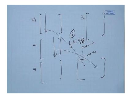
Whereas in LTE by virtue of having code books it is still possible to multiple users. So, that in a fashion, for instance one could choose a different columns of these different matrixes and form 1 new matrix which is using columns from different users in such a way that different users data or these streams they do not interfere with each other and in this wave in the signal is transmitted across to the users would have almost interference free communications.
