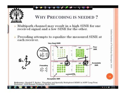
So, that we are able to get some better signal quality and reduce the variability of the channel moving forward this particular slide gives a brief in intuitive explanation that why we are going for pre coding basically by pre coding we are sending this signal x 1 over multiple paths and s 2 over multiple paths just like similar to diversity.
