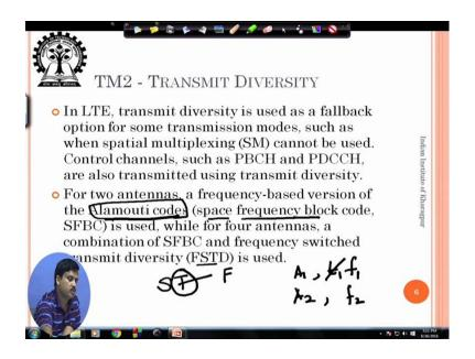
So, it allows transmit diversity. So, what this particulars slide tells you have to run quickly through this is basically, we are studied Alamouti in the time domain right. So, we have studied at in the space time block coding, whereas, here it is used in the space frequency block code the difference here is this time that we have studied is simply replaced by frequency.
