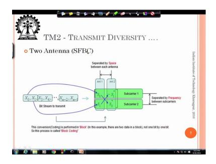
You can always use m r c at the receiver that is always possible. So, this particular slide gives you brief overview how is done. So, here you see clearly there is antenna 1 antenna two. So, here is sub carrier 1 sub carrier two, but we have studied time 1 and time 2, right. So, we move forward.
