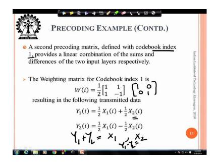
So, basically we would write as s times w times h is what is being transmitted is been received along with noise. So, this can be used to provide an identity matrix to indicate blast or any other combination to provide a particular pre coding moving forward there is another pre coding which is 1 of the simplest pre coding as shown over here and this is the code book index 1 here the code book matrix is like 1 minus 1. So, in the previous case it was 1001.
