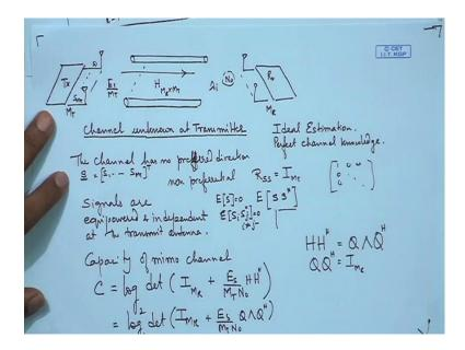
So, when we look at MIMO we have drawn these pictures several times before indicating MIMO system. That means, this is the transmitter and we similarly have receivers with multiple antennas, and we have indicated that there are MR is a variable use for indicating number of receive antennas MT is use to indicate the number of transcript antennas and H is the channel matrix which of dimension MR cross MT we have done on this expression we have also looked at the expression of capacity.
