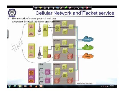
Moving on further if we take a look at the typical cellular network there is a base station there are subscriber modules. So, this part of the network which is having the mobile phones and the (Refer Time: 10:43) station is typically part of the access network. In case of mobile telephoning it is also known as the radio access network.
