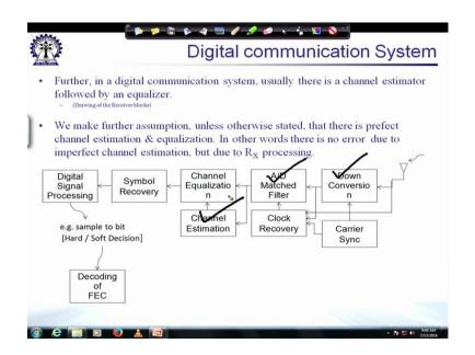
We move on to the next important assumption about digital communication systems that we make. Typically in a digital communication system we have the channel estimator, because between the transmitter and the receiver there lies the channel. So, as we have just drawn in this figure between the transmitter and the receiver there lies the channel which is for us to workout.
