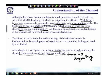
For example, if we take the example of MAC, the medium access controller is usually one of the most important entities which control access to the medium the physical medium. When MIMO was introduced MIMO allows two or more users to be connected simultaneously. This is one of the important things that we will see in the course.
