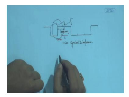
In other words if we considered the symbols in baseband to occupy a certain symbol duration and so on, so we take match filtering for rectangular pluses typically we will be having the integrate and (Refer Time: 23:47) circuit which can be graphically represented through an integration followed by a dump operation which goes on happening for every symbol duration and the values are read off at the peak where the symbol duration ends.
