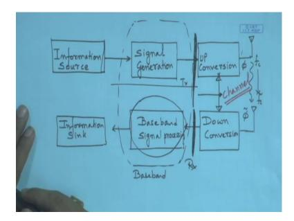
What we mean is suppose we have an information source. This could be analog or this could be digital, if it is analog we will assume analog to digital conversion. It goes on to the section of signal generation followed by RF section or up conversion and then finally into the medium. At the receiver we have the reversing happening; we have the down conversion followed by baseband signal processing. Once the signal has been process it can be given back to the information sink.
