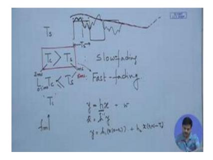
So, with this we go into a very important definition of our study. If suppose we have t s as the symbol duration. Symbol duration means we talk about digital communication system. So, in a digital communication system supposes we are sending symbols which are like this and so on. So, let be this be the symbol duration. So, if the coherence time as we measured in multiple ways is larger than the symbol duration. So, what will happen?
