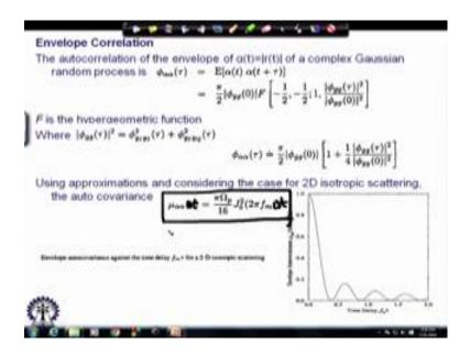
So, with this we move on to see what happens to other properties of the signal. So, what we would lastly like to see is the envelope correlation. Envelope correlation is basically the correlation of alpha alpha t basically we talk of phi of alpha alpha delta t which is equal to the expected value of alpha of t times alpha of t plus delta t where, alpha of t is equal to mode of h t.
