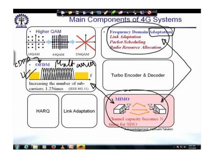
If we look at the main components of 4G again we see the prominence of MIMO techniques coming into picture along with frequency domain link adaptation or frequency domain radio resource allocation. So, these two together forms the major gain provider of 4G systems compared to earlier communication systems. What we see over here is adaptation is one of the major things that were supported to 4G systems. Of course, we have OFDM this is not mentioned because this is so well known today.
