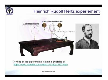
Moving on to further what we have is the experimental setup which Heinrich Hertz used. What I have given below is the YouTube video link which real demonstrates in a nice way how this experiment was performed. What you have done was used an oscillator as indicated by the mouse pointer here, and he has used a spark gap in between where they used to be occurrence of sparks due to be oscillation.
