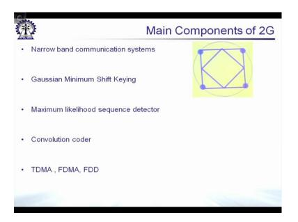
If you now take a look at the 2G the important components of 2G were narrow band communication systems, Gaussian minimum shift keying was used, maximum likelihood sequence detector was used, time division and frequency division multiple access and FDD systems were used.
