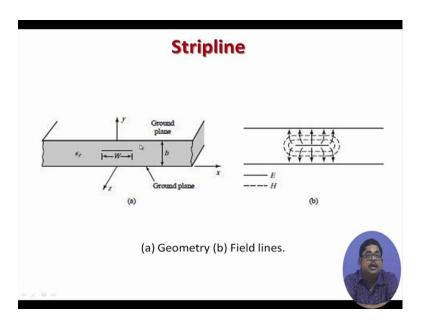
The first we will see is called a strip line. Now strip line is the geometry shown here, you see that there is a ground plane on the top, there is a ground plane on the bottom and between the ground planes there is (Refer Time: 02:06). But there is another thing sandwiched in the inside this (Refer Time: 02:16), that is a metal. So, there is a, this metal which is infinite in another transverse direction; that means, if we call it y sorry
