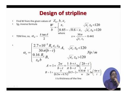
So, now you people have if any design strip line is to be designed then the job is actually to find the width from the given value because generally the characteristic impedance of any transmission line is specified. So, strip line what characteristic impedance is required that is specified and b is the separation of the 2 ground planes and epsilon r these will be given. So, from that by putting into those formulas we will have to find out what is W.
