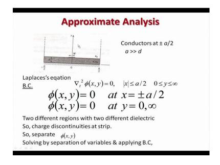
Now, approximate analysis follows like what we have done for the strip lines. You put Laplace's equation inside this confined zone. So, again there will be this boundary condition that in the side walls the potential function should go to 0 and the top and bottom potential function goes to 0. So, again there is that is this micro strip will have some charged distribution.
