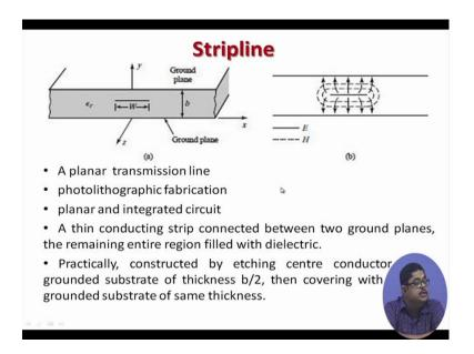
Now, it is a planar transmission line; obviously, you see that the whole structure is plane or not that like that 3D things like wave guide and (Refer Time: 4:35) etcetera by photolithographic fabrication it is made. As I already said that since it is planar and it is amenable to integrated circuits so microwave integrated circuit we used this strip lines as the transmission lines.
