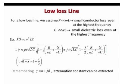
So, propagation constant gamma of a lossy line will become like this and we have seen in your transmission line classes that R plus omega L also like that if you do it becomes this. Now, for a low loss line because we will have to use it so, in our use it will be low loss line means small conductor loss even at the highest frequency.
