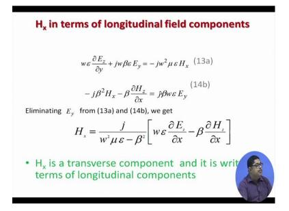
So, here we have shown that if you eliminate then Hx from these two equations 13a and 14b and if you eliminate y from 13a you get Hx. So, now, by this we can know that Hx is a transverse component and it is written in terms of longitudinal component.
