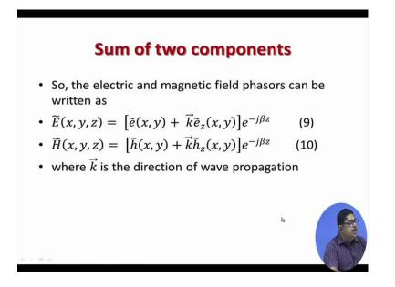
So, we can write these phasors which will be having E x, y, z that is breakable into this is the transverse component plus k ez ex y then we know, but this is the two direction and what is the z variation of this electric field e to the power minus j beta z because the wave is propagating in the z direction.
