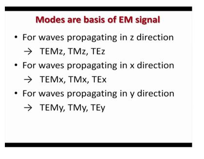
Modes are basis of EM signal and I have already said that all EM signals are basis set of the modes. So, if we have waves propagating in z direction the basis set we call TEM to z, TM to z, TE to z.
