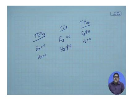
But now I am trying introducing Te wave, it means that the electric field is transverse. Electric field transverse means it will have Ez is equal to 0 and it does not have magnetic field transverse.
