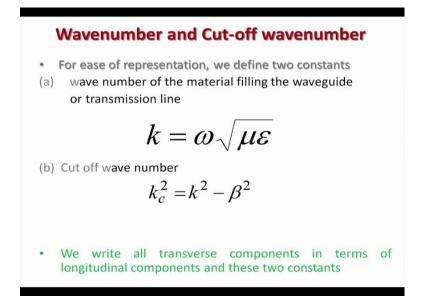
So, that also depends on the materials and these will give some name and that name or wave number and cut off wave number, wave number already we are familiar that is the propagation vectors magnitude so that is, omega into this and will also define a cut off wave number k square minus beta square. So, we write all transverse components in terms of longitudinal components and these two constants.
