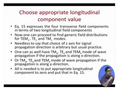
So, this equation 15 is the part that we have manipulated somewhat and got you. So, choose appropriate longitudinal component value, equation 15 expresses the four transverse will components you can put the TEM, TEz values needless to say that choice of z axis for signal propagation direction is arbitrary, but usual practice one can as well have x directed propagation etcetera, all is needed to put appropriate longitudinal component to 0 and put that in equation 15.
