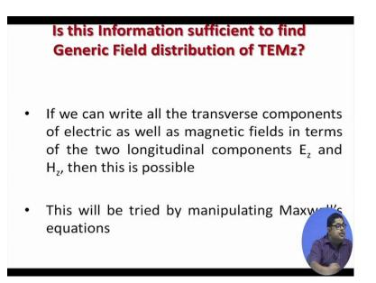
Now, is this information sufficient to find generic field distribution of TEM z? The answer is yes if we can write all the transverse components of electric as well as magnetic fields in terms of the two longitudinal components Ez and Hz, then this is possible because by being TEMz, we know the values of Ez and Hz.
