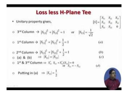
Now, you put the loss less condition that is unitary property. So, by that to proved that really half power is going and. So, and one the mismatching the 2 ports 1 and 2 their
