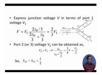
Now, this junction voltage in terms of port 1 voltage you can easily write. If this is V 1 this will be r plus this, 1 is small z by 2. So, if you do that you can easily relate V and V 1 that we have done here. So, V is equal to two-third V 1.
