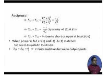
And then we calculate some values then what are the S parameter value. So, we got this thing, that it is a reciprocal when power is fed at port 2, so infinite. So, we calculated this S 23 and S 32 they turned out to be 0.
