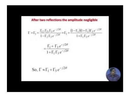
So, if you do that finally, we will see that gamma after two reflections finally, you can sum that geometric series and it becomes like these. So, the thing is mainly the first reflection is very important and also that second reflection means that one transmission going to load coming back, these two are important others are there, but the value is falling. So, mainly these two determines the steady state.
