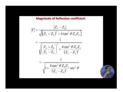
Now, this is what is the previous expression was the complex reflection coefficient. Now, we are interested in mismatch that is based W r. So, that is depend that is scalar quantity. So, the magnitude of the reflection coefficient is sufficient to get W r, that is why we take the magnitude of the reflection coefficient, and that turns to be these ultimately you will see that we some mathematical manipulation it become a some trigonometric relations.
