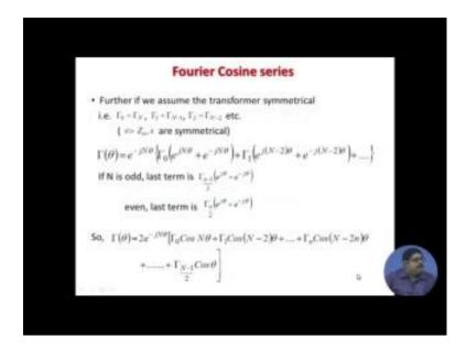
Now, we also assume two more things, one is the transformer is symmetrical, symmetrical in the sense that the reflection coefficient at the two ends the remaining is suppose I have multiple sections.
