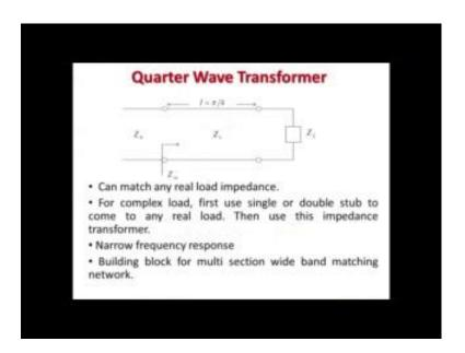
The element by which that is done can be done, one of the simple schemes is called Quarter Wave Transformer it is basically a section of a larger scheme. So, in itself it is not a broadband transformer, but with it you can achieve any broadband design that is important. A quarter wave transformers is shown in this slide, it consists of quarter wave means the length of this is lambda by four not pi by 4.
