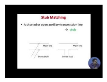
Now, the impedance matching network if there is a power transport going on in the main line that is called main line, and for impedance matching we use some auxiliary transmission lines. Now, that transmission line may be shorted or opened that are called stub. So, I can have an open stub or I can have a short stub. Now, as you see that there is a main line from that the stub can be connected either in shunt that topology is shown or it can be a series stub also.
