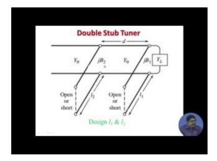
So, people come up with a double stub tuning where the 2 stubs are used not 1 stub, but the distance between the stubs that is called d that is fixed this 1 is fixed. So, stub positions are fixed load immediately connected to the first half then there is d that also fixed connected to second stub. So, what is the design? Design is what is the lengths of these stubs. So, that from here you see a matched design.
