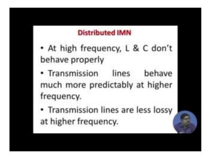
So, that design is called distributed impedance matching network. Transmission lines are less lossy at higher frequency. So, they are used for this impedance matching network.
