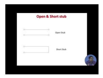
The other end is left open whereas, a short stub the end which is not connected to the transmission line that 1 is shorted then it is called a short stub
