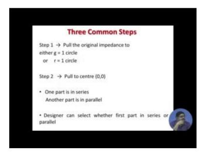
So, if you summarize the common steps in all these step 1 is pull the original impedance to either g is equal to 1 circle or R is equal to 1 circle which 1 is appropriate depending on your position then by the next part of the component you get pulled to the centre. So, the first part of the component that brings you to either R is equal to 1 or g is equal to 1 circle and the second part brings you to the centre. So, 1 part will be always in series
