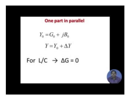
Now, similarly the branch may be in parallel in that case the new admittance will be the old admittance plus delta Y and for L and c the conductance change will be 0.
