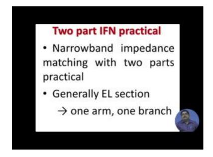
So, narrow band impedance matching with 2 parts is more practical generally that is called 1 section actually 1, but to pronounce sometimes it is e 1 also called. So, basically in an e 1 section you have 1 arm 1 branch; that means, 1 series element 1 parallel element
