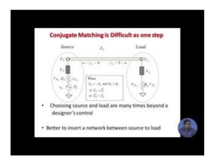
In many practical cases that conjugate matching, we have seen that it is ideal of impedance matching if you can do conjugate matching between source and load you can do many things. So, achieving both this gamma S that means, source reflection coefficient 0 and also the load reflection coefficient 0 by making the source and load impedance conjugate to each other, now that always is not at the hand of the designers.
