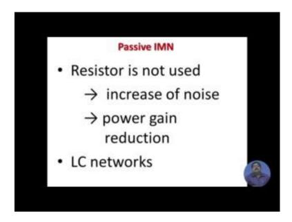
So, in passive IMN again you can make it with R 1 c, but resistor is generally not used again that it has some power dissipation. So, that is why if you can avoid, it is good also resistor again has a bit of noisy device. So, generally resistor is not used for passive integrated matching networks. So, mainly passive IMN by that we mean LC networks composed of either L or C.
