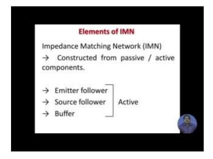
Now, this impedance matching network, IMN they can be constructed from either passive or active components. Now, there are good impedance matching network, they can be done with active elements like transistor based emitter follower source follower buffer there the active elements bits IFM.
