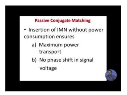
Now, you ensure the maximum power transport, no phase shift in signal voltage here also.
