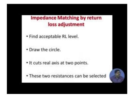
So, impedance matching by return loss adjustment, find acceptable R 1 level draw the circle it cuts real axis as 2 points. So, those 2 resistances at the extreme points beyond which you can need not go.
