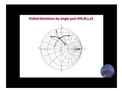
Now, the impedance matching network is either adding either an R or L or C any of them a single one. So, if it is a single element L, it is a movement in the clock wise direction, if is A C S it is in the anti clockwise direction. So, you see various pool directions here
