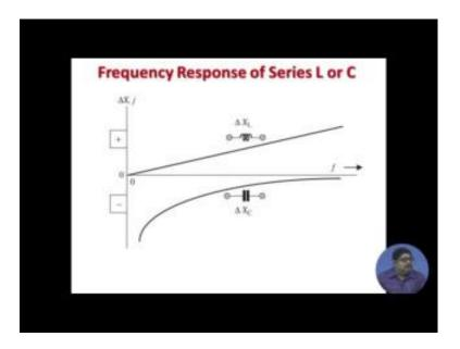
Now, frequency response of a series L or C you can see that that varies like this is the frequency response. So, for inductance it is linearly varying for capacitance it varies not inductly, it is a hyperbola type of variation and you know this this frequency response is known.
