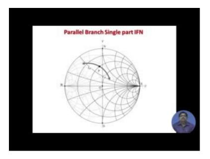
Now, in smith chart this means from the point P from this point P if I have a parallel branch of inductance. This means I am going in the anti clockwise direction whereas, for A C P parallel capacitor in parallel branch I am coming clockwise. Now, that means, that in this the previous 2 pictures I have put here. So, the point P you try to see this point is the point P. So, there is an impedance.
