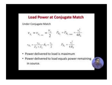
So, if conjugate matching occurs; load power at match. So, under conjugate match, we know what is the voltage developed at the load, that you worked out because that time no reactive part in the total reactance is 0. So, voltage, but two equal resistances this R S and R L equal. So, half of the source voltage is across R S half of the source voltage is across r l.
