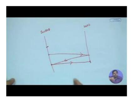
Suppose; if I look at these that this is the load this is load and this is source, then you see that suppose now I am here. So, one wave has come just T d time before. So, this source has delivered and it has come here, but this time also another one is coming, 3 T d time before there was another wave.
