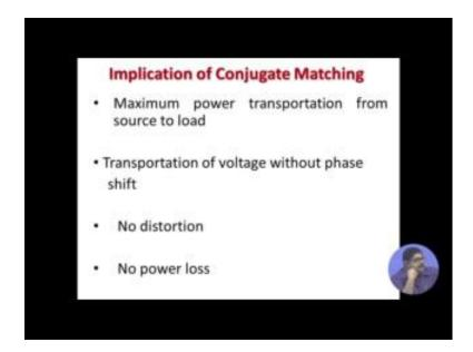
So, what is the implication of conjugate matching one we have seen that it is maximum power transportation from source to load, transportation of voltage without phase shift also under that case the gamma l, load deflection coefficient is 0 gamma S is 0. So, no distortion will be there no power lost will be there.
