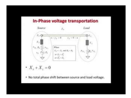
Now since, the total reactance of the whole network under conjugate match is 0. So, we can say that there is no phase shift between the source voltage and load voltage. So, this is call in phase voltage transformation.
