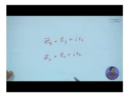
So, we can always write the Z S is equal to R S plus j X S. Similarly in the load side we have R L plus j X L and, across the resistance R S there will be a voltage drop we are calling that v R S across that resistance or in that resistance there is a power drop or power dissipated that we are calling p r s.
