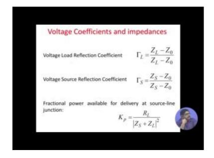
Two reflections at source and load changes phase by 360 degree. So, no phase change with all these things we can now see that, voltage load reflection coefficient this is well known in last week's lectures also we have used these that the load reflection coefficient will be the load impedance minus the characteristic impedance of the line by oh again those same mistake Z L plus Z 0 it will be. Sorry! Please see in here last time also I did not correct it.
