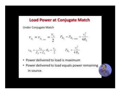
So, power we can calculate that will be the v s square by 4 r l. So, power delivered to load is maximum power delivered to load equals power remaining in source. That means, in the as per the source resistance what is the power the same power you can deliver to the load not more than that.
