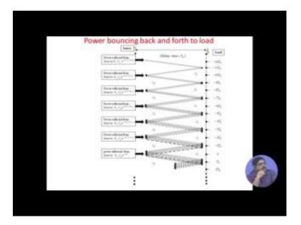
Now, actually what happens power is continuously bounces to and flow from load to source? So, let us try to see that suppose the source and load they are separated by a distance and the travel time of the wave to that distance, let us call t d. So, this; the wave
