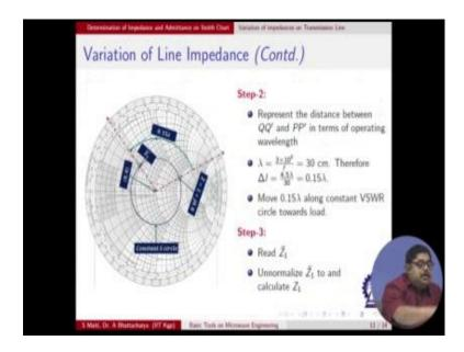
So, step two, since the smith chart movement markings are in terms of lambda so you find out that in the problem it was said 4.5 centimeter, but that is how many lambda, so that you need to convert. As shown here that lambda for your 1 giga hertz frequency, so it is 30 centimeter. Simple calculation the 3 into the speed up light, 3 into 10 to the power 8 meter per second this are speed up light by f, so that is 30 centimeter.
