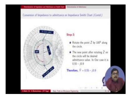
So, here we are showing that reflection means basically you are at the other end of the diameter. Now, we can read and you see that you are getting the correct value, so this shows that the procedures that whether you are in impedance smith chart using or admittance smith chart using you will be able to plot anyone correctly. So, these four I think examples.
