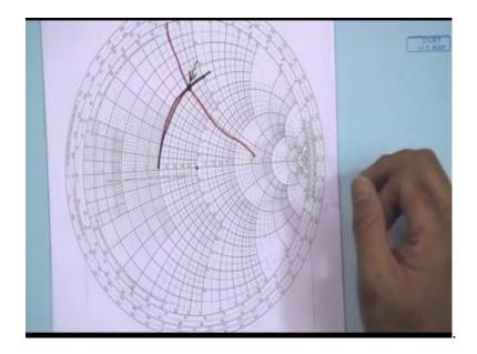
So, this one is that and 0.5 by thing is this circles sorry, so these intersection points somewhere here is our desire that point. So, by this I can locate any impedance if I want to locate on the smith chart this is procedure.
